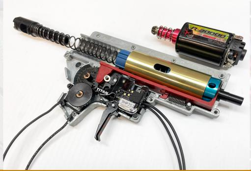
"MY CONCERNS ABOUT THE MOTOR GRIP PROVED SPOT-ON; WITH THE LARGER 16 AWG WIRES FROM THE TITAN, IT TOOK A LITTLE FIDDLING, CAREFUL POSITIONING AND LIGHT MODIFICATION OF THE MOTOR PLATE TO MAKE IT CLOSE UP PROPERLY."
