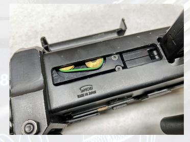
pushes the BB's into a single-track channel that's been machined into part of the gearbox shell. This channel curves towards the back of the gun before making a vertical rise up and into the bottom of the hop up chamber, which is based off the Tokyo Marui AUG design. In this case, it has what I believe is a G&P
