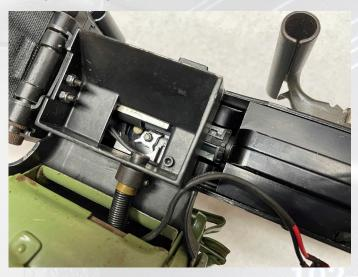
the BB's fall into a CNC machined feeder assembly that looks similar to a much abbreviated version of the Cyclone paddles found in the Tippmann A5 paintball marker. This "paddle" is powered by yet another RC servomotor that spins the paddle via an O-ring stretched over a brass pulley. The paddle then
