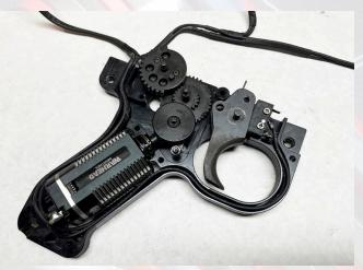
Inside we find an AUG length air nozzle, followed by a conventional mix of V2 compression parts and gears. The previous owner had at some point outfitted this with some old-school Super Shooter 32:1 gears and half-rack steel piston. It was also sporting a Guarder Bore-Up cylinder, silent-type mushroom piston head and bore up nozzle. There was also a V 3 tappet plate installed, which I assume was done on the mistaken assumption that since the AUG
