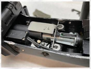
means the bottom pulley and O-ring are exposed to the elements or inopportune objects that might dislodge the O-ring from the pulley; the latter has actually happened once during an event. And let me tell you... it's a pain to try and reinstall that O-ring in the field without tools and a dental pick handy!
