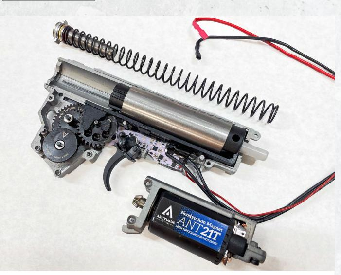
made me concerned this was using a slim type motor, which have been somewhat problematic. Fortunately my fears were allayed, and this slimmer profile is accomplished by using a G36-style motor cage to house a conventionally-sized motor.
